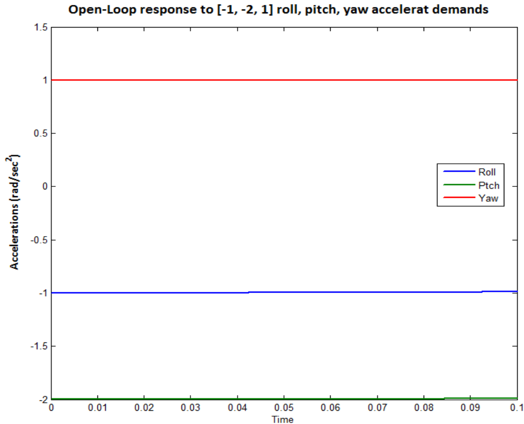
Figure 5.6b Response of the Open-Loop System to Roll, Pitch, and yaw Acceleration Demands
