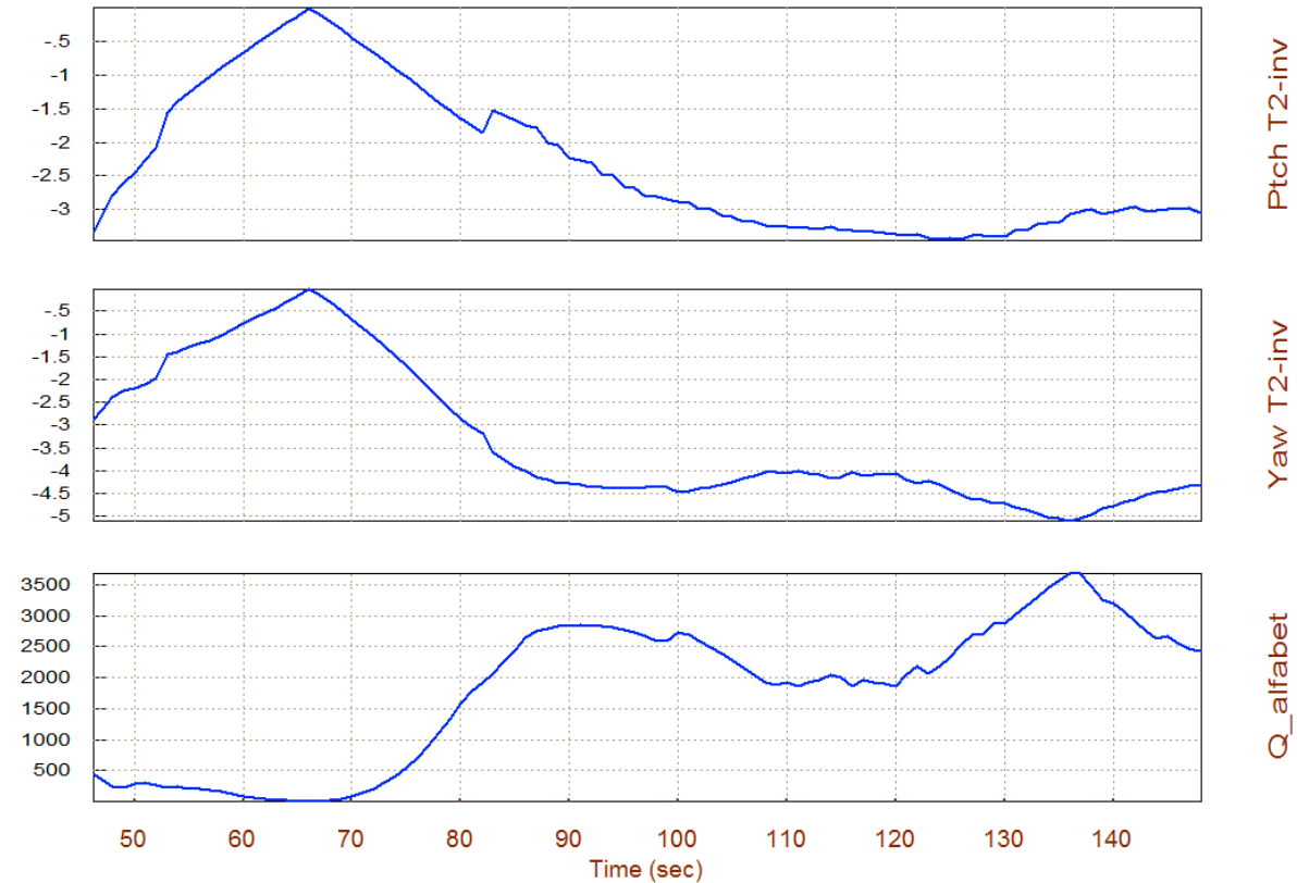
Short-Period (w)/ Time-to-Double-Ampl-Inverse (/sec), Q_{\alpha\beta} (deg-lb/ft 2 )
